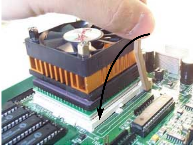
Figure 8. Locking the CPU upgrade adapter into the ZIF socket
