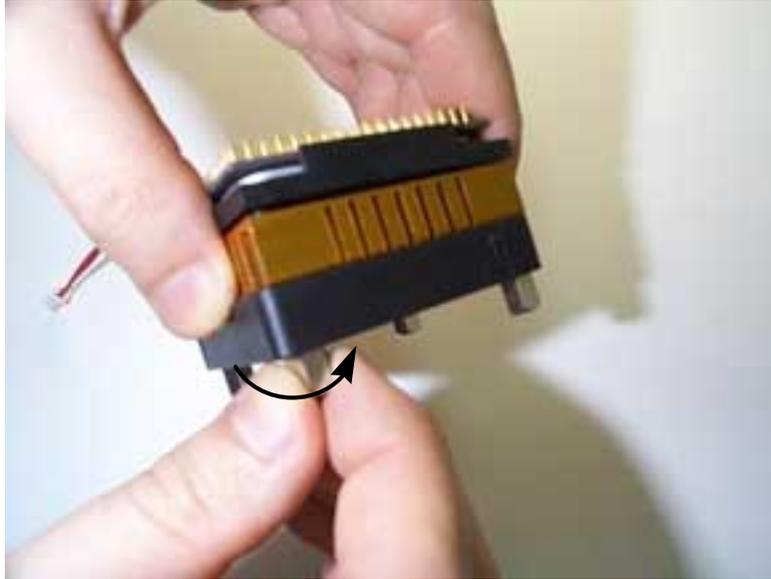
Figure 2. Tightening the hex nuts
