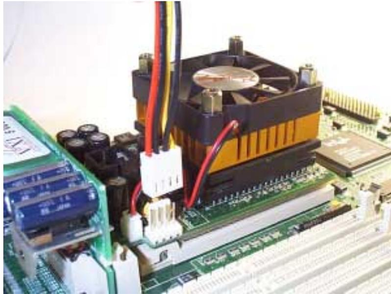
Figure 6. Connecting the power cable
